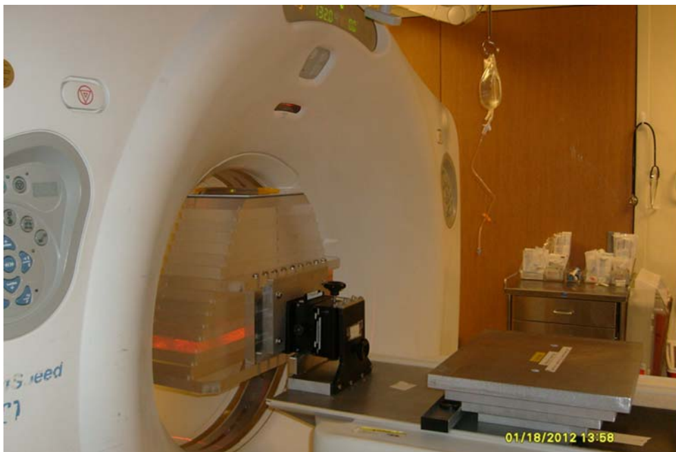
Figure 6.7 The whole PMMA phantom aligned in the scanner bore.
