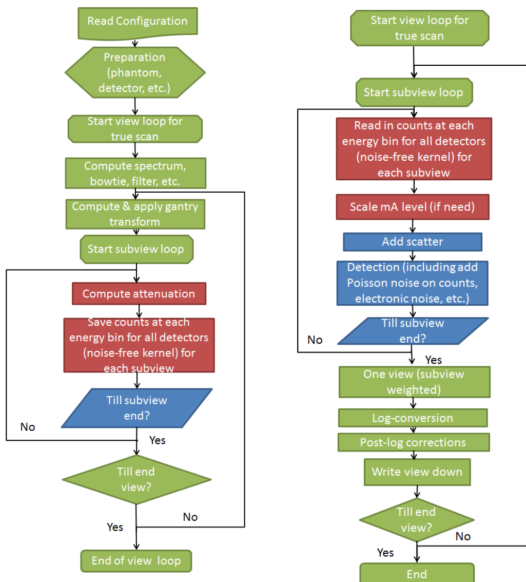
Figure 3.4 Modified CATSIM structure flow (Left: Part 1) for calculating noise-free kernel; (Right: Part 2) for calculating noisy simulations for different mA levels, and /or multiple realizations.
